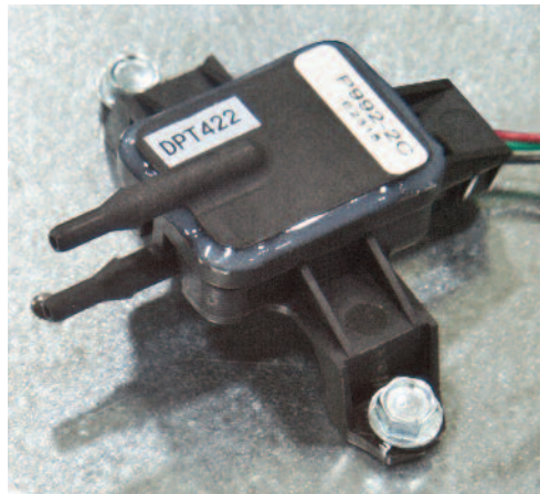
Figure 3 - Pressure Transducer in Electrical Box
